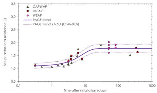
Fig. 20: Development of offshore PAGE piles’ total resistance setup with time.
