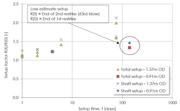
Fig. 3: Setup factor (total resistance and shaft resistance) versus setup time: Los Angeles Export Terminal piles.
