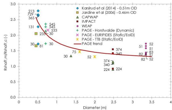
Notes: 1) PAGE data combined with other case histories, 2) Normalisation using Unified resistances, 3) Labels indicate number of days after driving when testing was performed (setup time)
