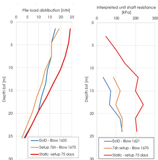
Fig. 15: Axial load distribution and interpreted unit shaft resistance for Trans Tokyo Bay pile tests on Pile P8.
