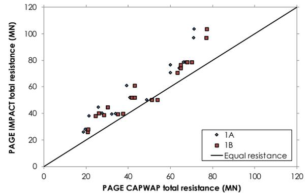
Fig. 5: CAPWAP – IMPACT comparison of total resistance (1A without radiation damping, 1B with radiation damping).
