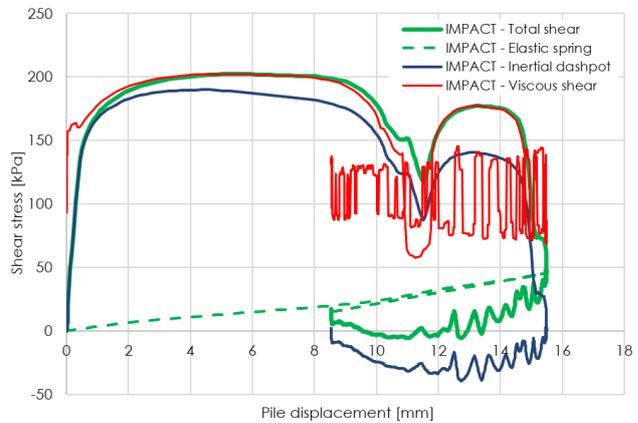
Fig. 13: Shear stress v pile displacement for IMPACT soil model.
