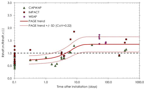
Fig. 24: PAGE offshore pile setup trends normalised by Unified total shaft resistance estimates
