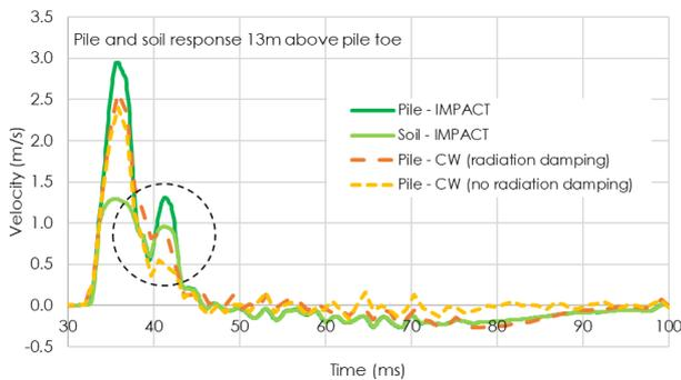
Fig. 11: Pile and soil velocity response.
