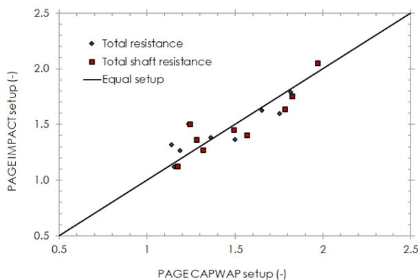
Fig. 7: Comparison of setup factor derived from CAPWAP and IMPACT.
