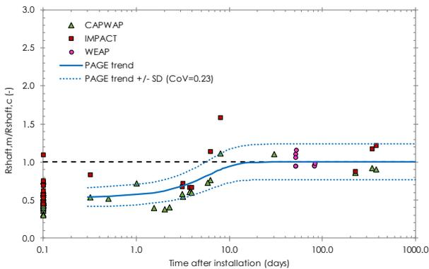
Fig. 25: PAGE offshore pile setup trends normalised by ICP total shaft resistance estimates.
