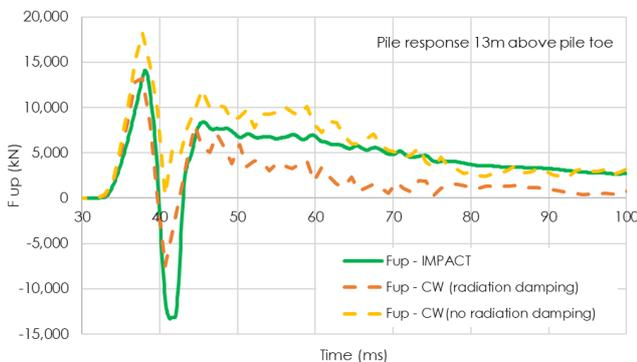
Figure 12: Upward traveling force wave
