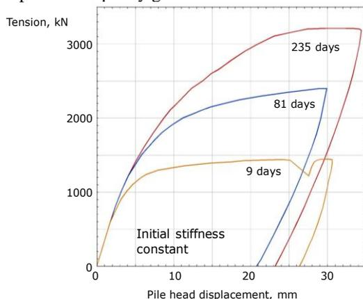
Fig. 1: First-time static tests on identical piles driven at Dunkirk, after Jardine et al (2006).
