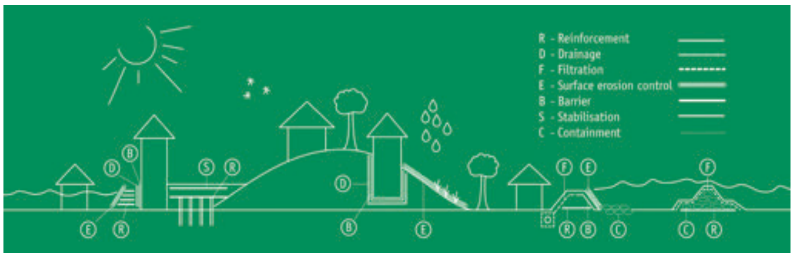
Figure 11 – Cross-section illustration of climate adaptation with multiple options for geosynthetic applications.
