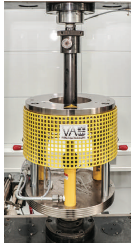
Figure 5 – EN ISO 12236 Geosynthetics – static puncture test (CBR test) - Simulation of the penetration of a stone through a geotextile for classification of the robustness class.
